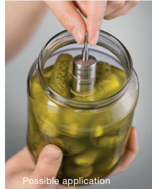
Temperature measurement directly in the food: testo 191-T1
